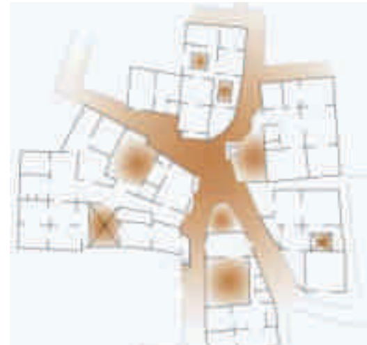
The incidental spaces resulting from the organic street pattern are raised as platforms used as spaces for community interaction
